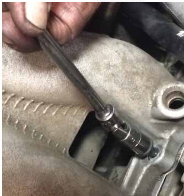
Using this tool, a 10 mm swivel socket with extension works ideally.
