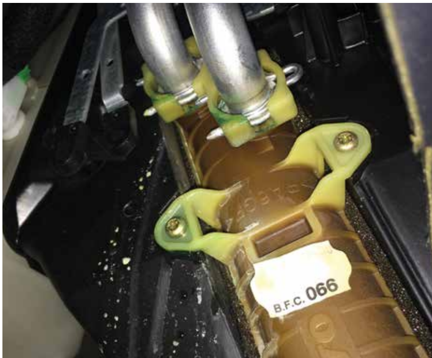
Hard pipes going into the heater core
