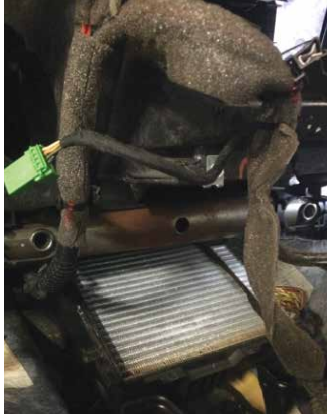
Here is a 2006 Volvo S40 heater core in dash, exposed.
