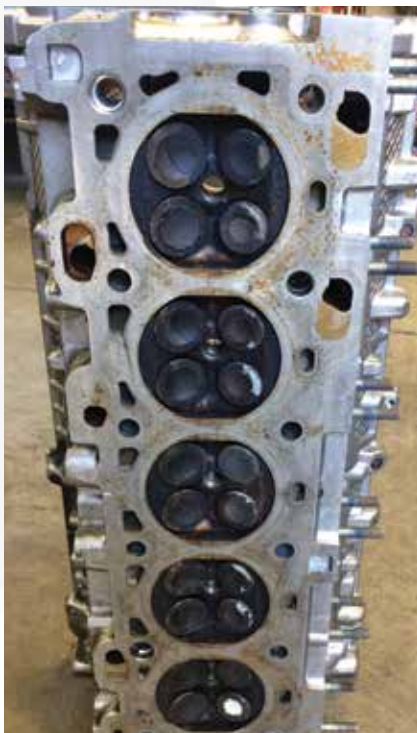
Cylinder head removed
