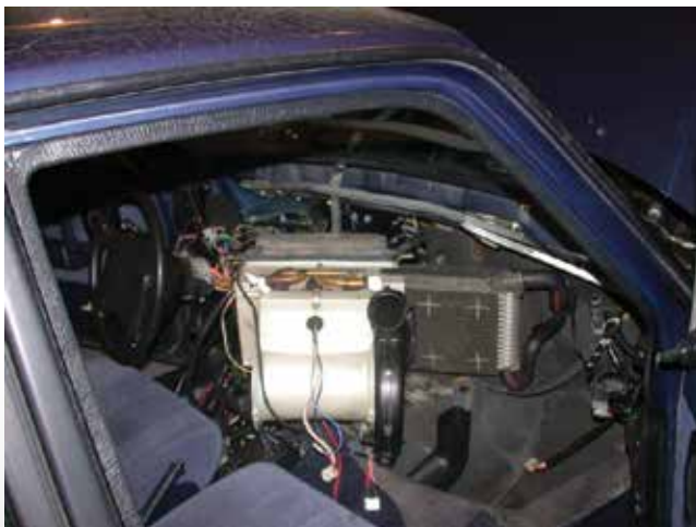
Heater core box from 240 modules
