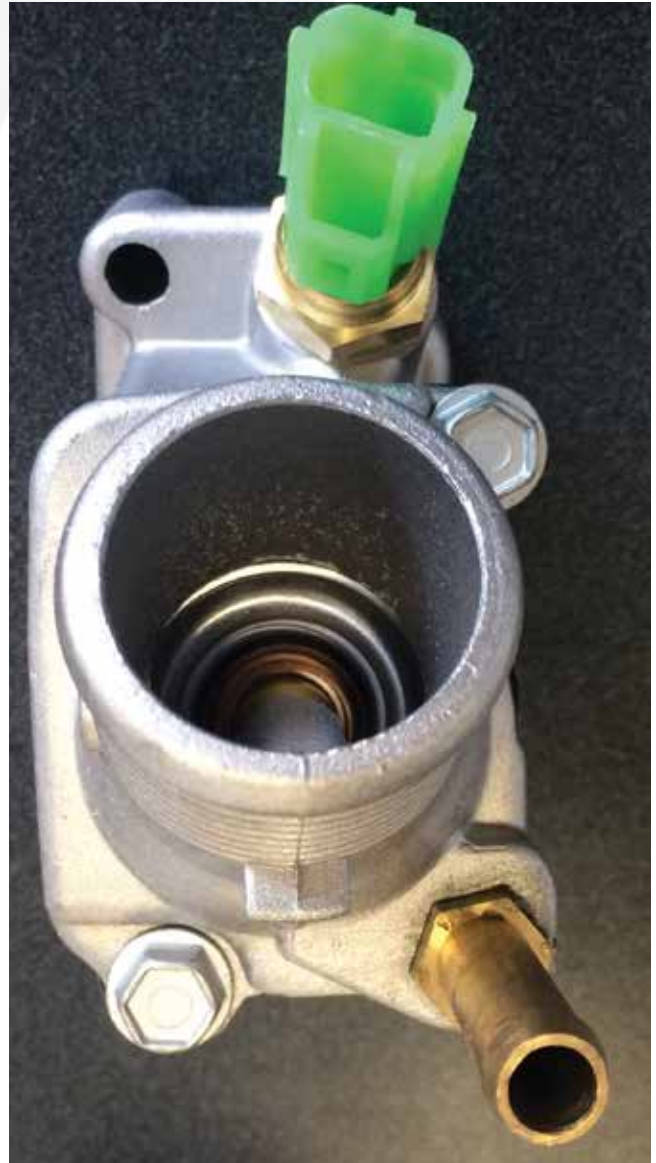
The coolant temperature sensor is right in the thermostat housing as shown.
