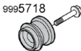
Tools for installing cam seals
