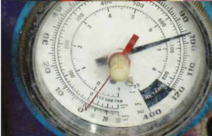
This image shows an inactive system with refrigerant pressure even on both low and high sides.
