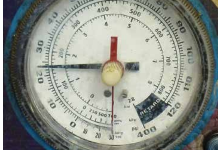
This is a great pressure drop reading from a properly operating A/C system.
