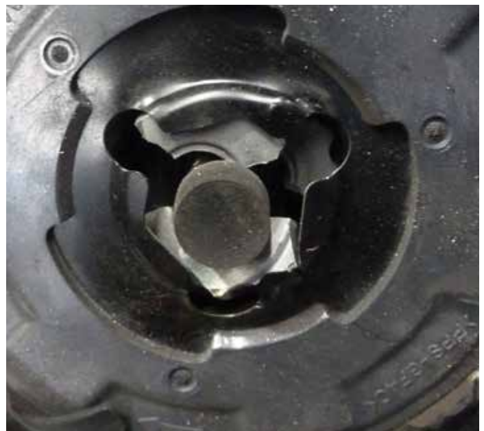
This compressor was exhibiting a clunking noise.
