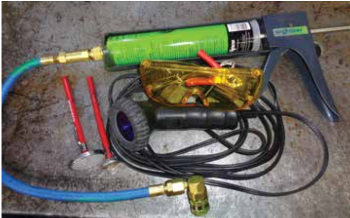
Dont forget the basics! Thermometers for the dash vents, and UV for the leaks!
