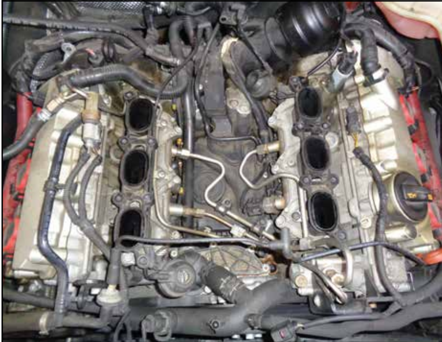
On this engine layout, the upper intake manifold must be removed to access most of the high pressure fuel system.
