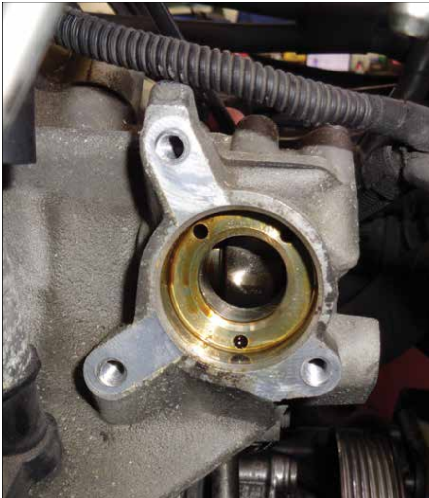
Always inspect the camshaft lobe for wear if the HPFP has been removed. It may be necessary to rotate the engine to find the high point on the lobe where most wear occurs.
