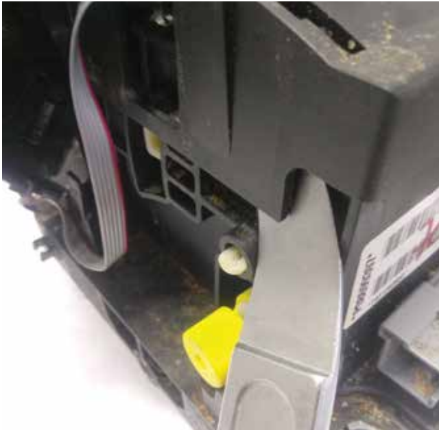
View of the broken rocker arm
