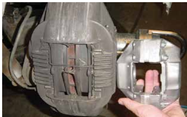
The 935 race caliper on the left dwarfs the "Big Brake" option of its day on the right.
