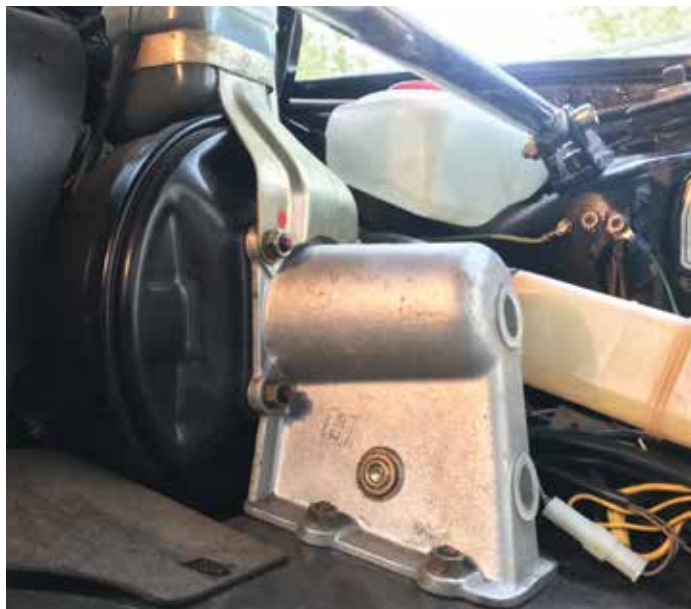
Difficult to access! The master cylinder is on the opposite side of the booster.
