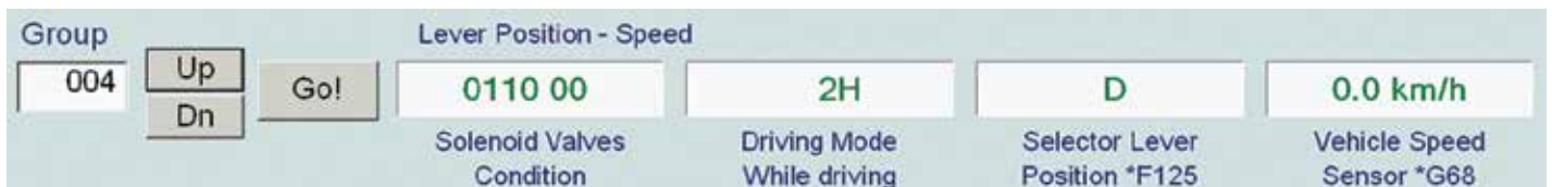
The fourth field is road speed. It is the output shaft speed at G68. With an open circuit and since the output shaft speed is not being read, the transmission sets limp mode, harsh gear engagement and starts out in 2H while in D with the wheels spinning at about 10 mph for a short period. The view is TCM group 004, field 4 and also found at TCM group 003 field 1.
