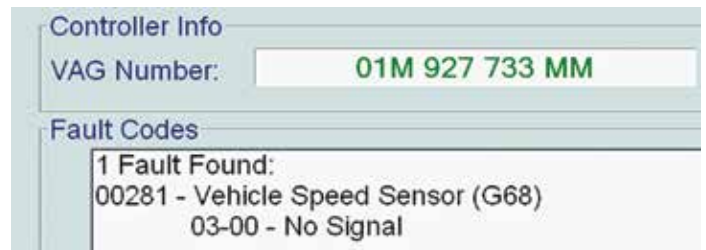
This fault was never recorded earlier and is immediate. The following images lead us to believe that the transmission was missing "road speed."
