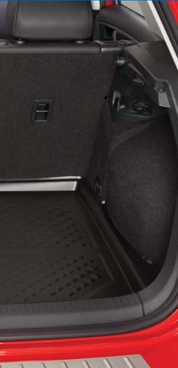
The trunk floor pan attaches to the rear cross member, frame rails, and rear cross panel (not shown) in this four-door 2015 Golf. It completes the enclosure and helps support the structural rigidity of the lower rear end.
