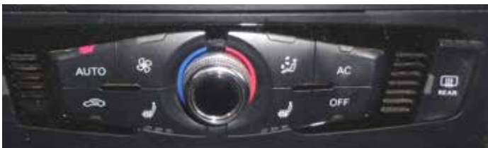
Audi has streamlined and simplified the climate control in this dual zone interface, integrating heated seats as well in the control surface.
