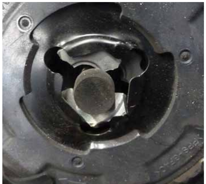
This compressor was exhibiting a clunking noise.
