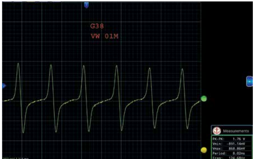
Engine running, in neutral, applying slight throttle will change the amplitude.
