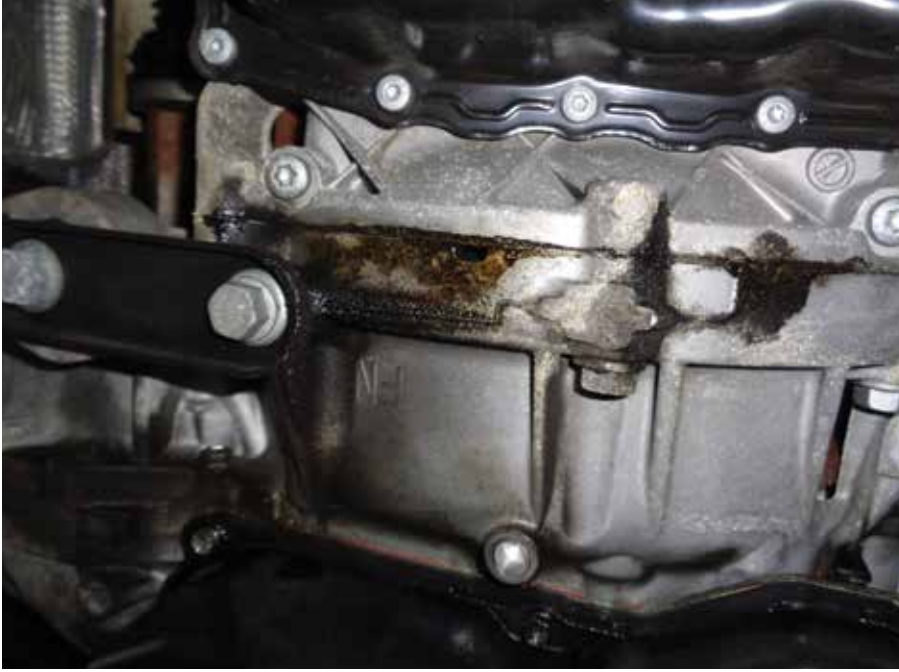
This is a clear sign of a leaking rear crank seal. This will lead to vacuum leaks and poor engine running if left too long.
