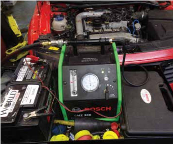
Having a smoke machine can make the difference between diagnostic darts and a definitive diagnosis.
