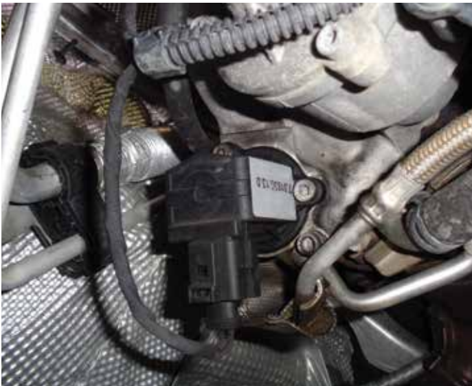
The diverter valve is easily removed and inspected from underneath the vehicle.
