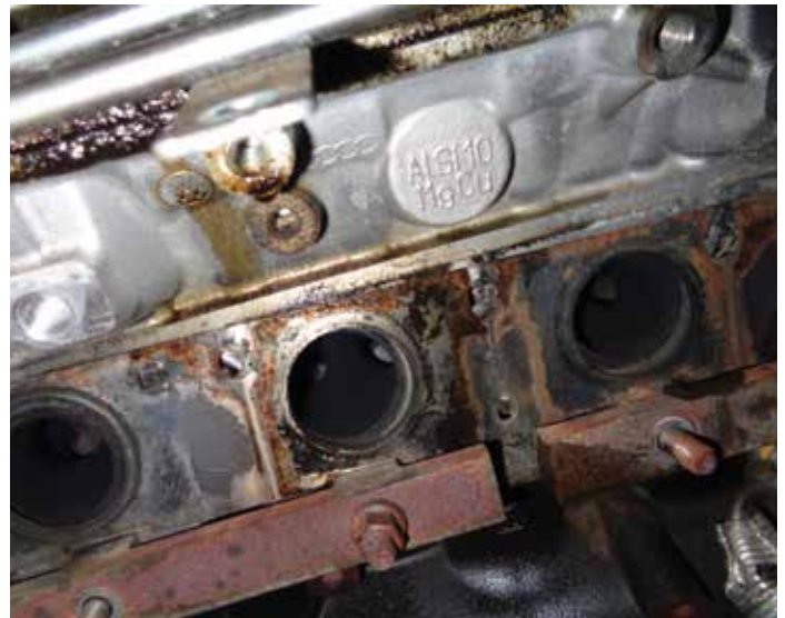
Access is particularly tight for the lower inner manifold bolts.
