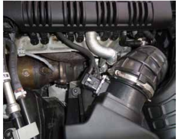
Turbo access from the top of the engine is limited.
