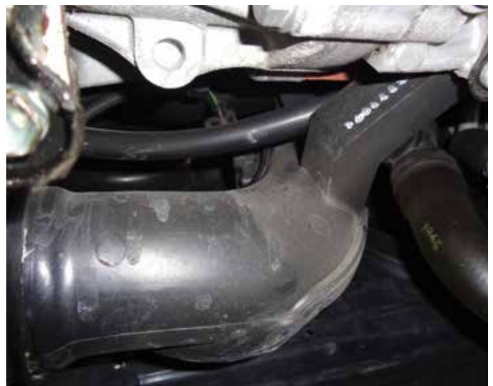
This boost pipe is commonly damaged during removal.
