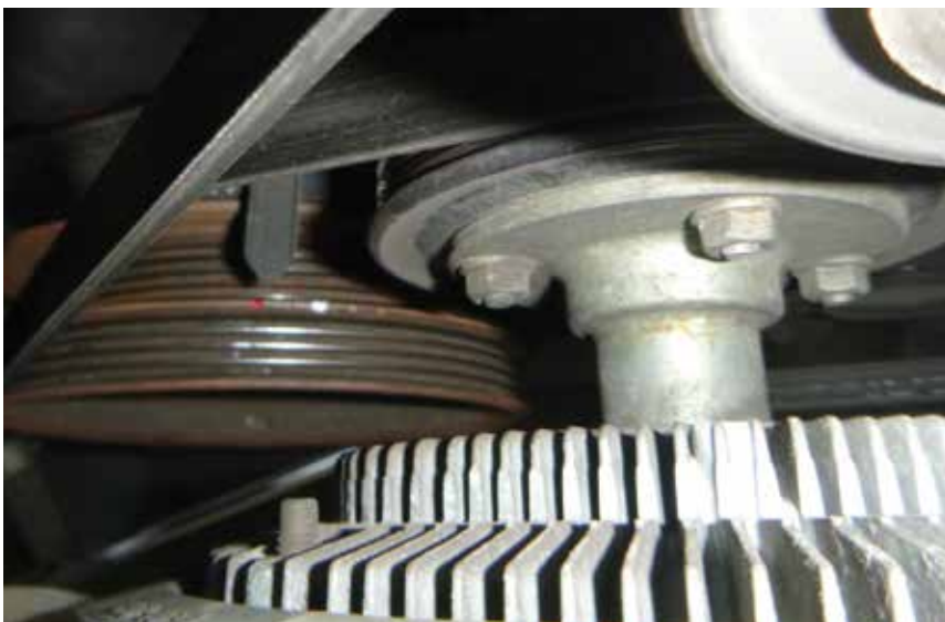
The red mark is at top dead center (TDC). This is where you want to be for a leak-down test. The white mark is 10 degrees BTDC which is typical for base timing. Each mark to the right is 5 degrees more advanced.
