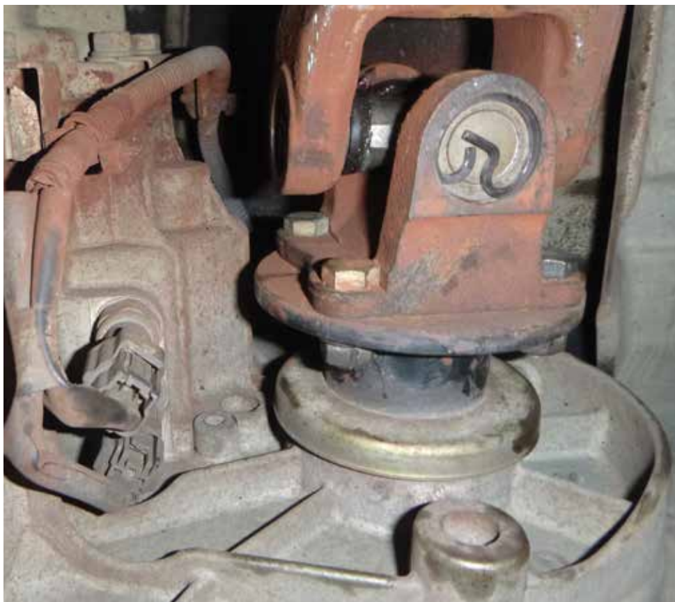
Simply looking at the transfer case we see the tell-tale blanket of rust indicating a failed Cardan joint. Catching these failures early can prevent further damage to the driveshaft yokes.
