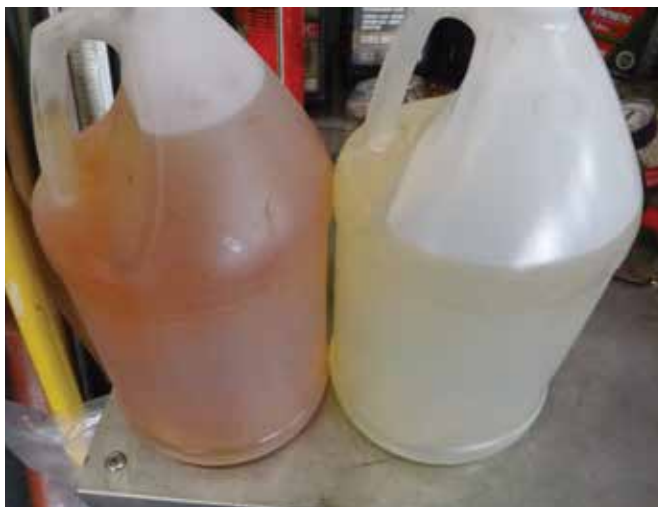
Fuel left to sit in the gas tank will eventually go bad and cause many problems, not the least of which is rough idle. The gas in the bottle on the left has spoiled and smells like furniture varnish. The difference is clearly visible compared to a bottle of good gas on the right.
