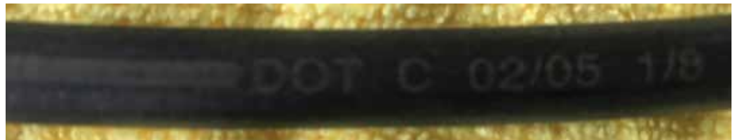
A close look at this photo shows the DOT stamp, certifying that it has been tested and meets minimum standards.
