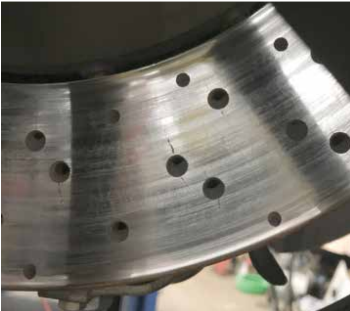
Some cracking is permissible! Refer to service bulletins for assessing whether a rotor with some cracking can be re-used. Standards are higher for cars used in competition.
