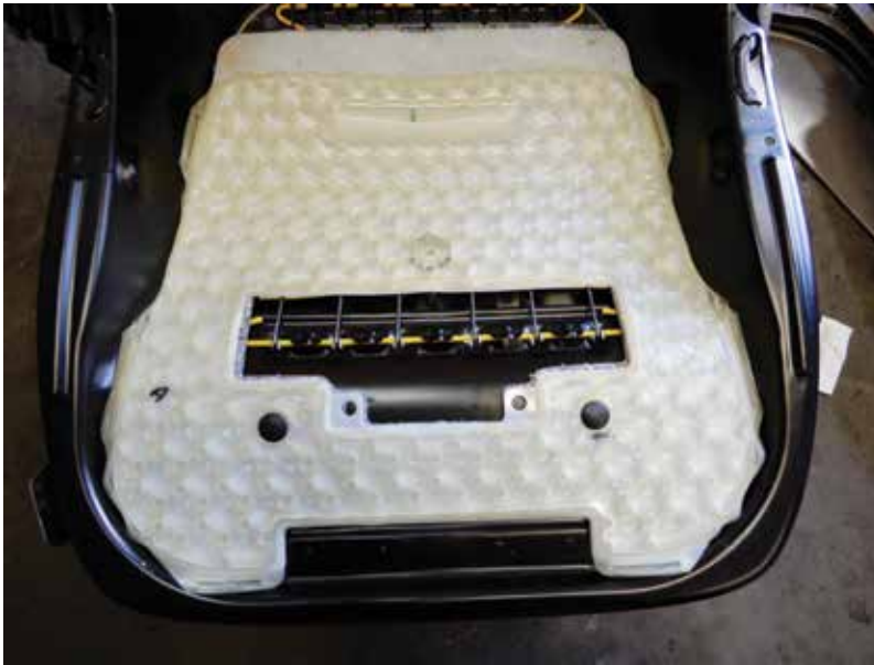
The Volvo weight sensor is located in the seat to calculate body weight.
