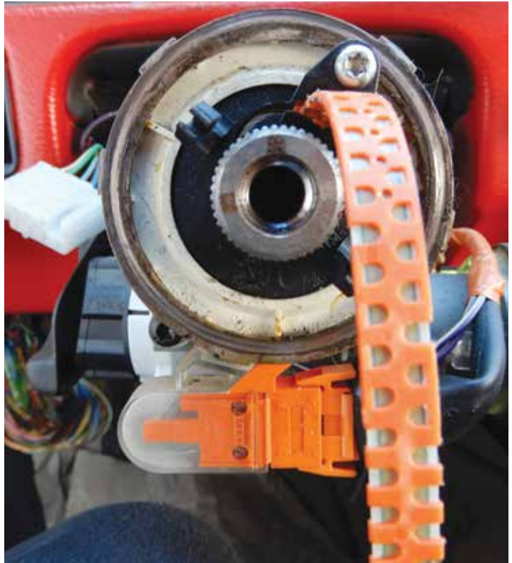
Volvo's clock spring or contact reel is found in the steering wheel and is also referred to as the steering angle sensor.
