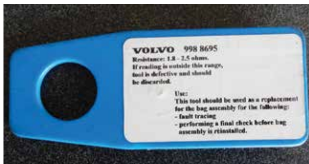
Resistor tool 9988695 takes the place of the air bag when diagnosing issues.
