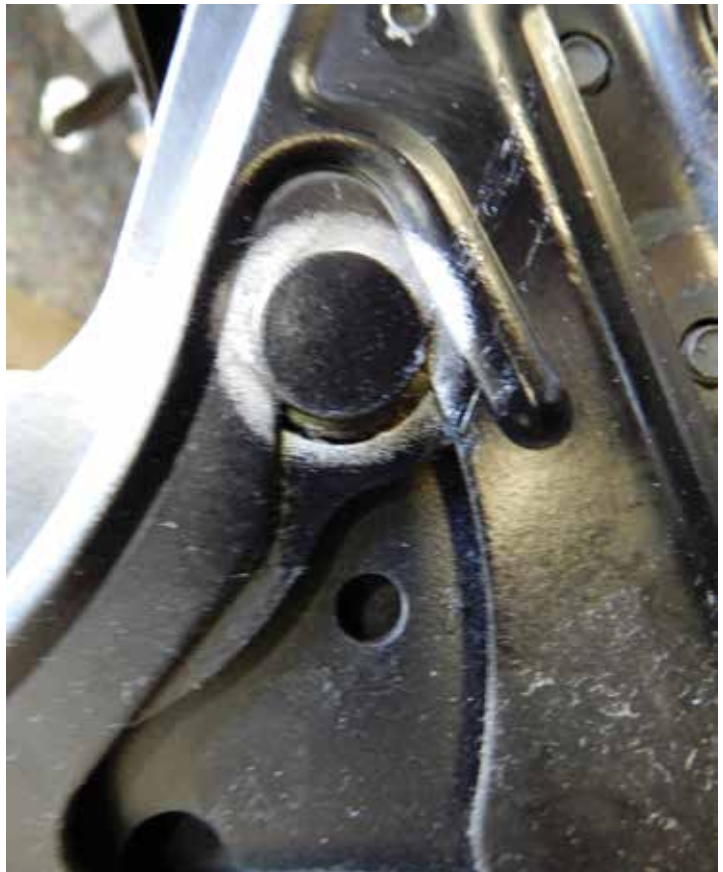
The whiplash rod needs to be replaced due to the gap opening.
