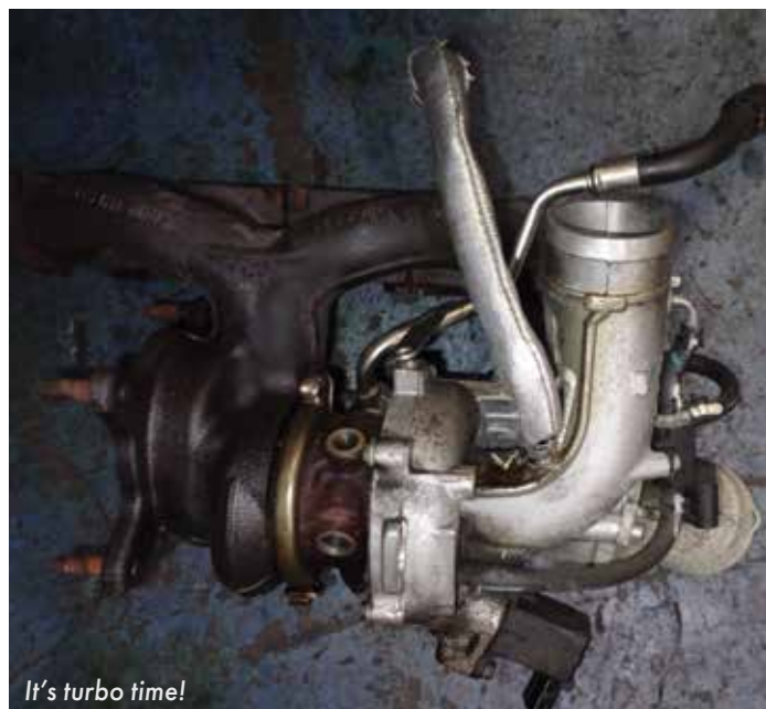
The actuator arm is only visible with a mirror or from underneath the vehicle when installed.
