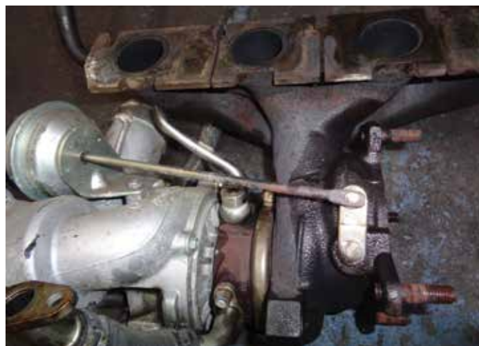
The actuator arm is only visible with a mirror or from underneath the vehicle when installed.
