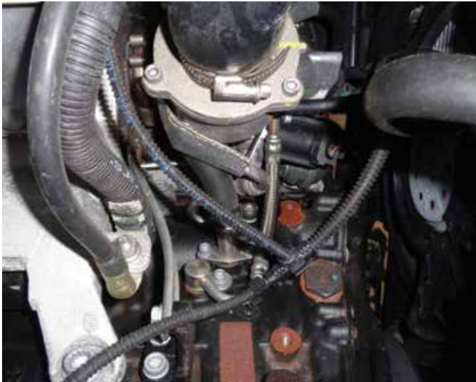
Be careful not to kink or damage any feed lines during turbo removal.
