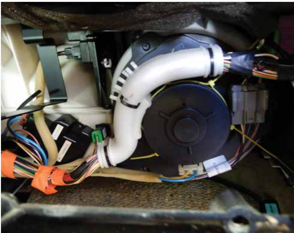
The blower motor and power stage are located behind the glove compartment in Volvo S70 models.
