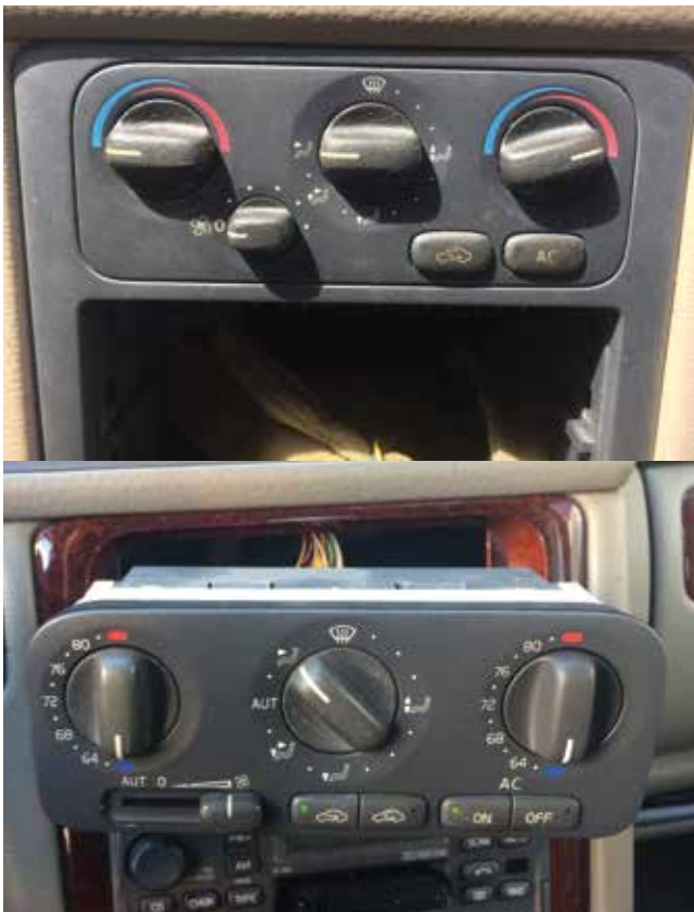
Here you can see the differences between the ECC and MCC front plate controls.
