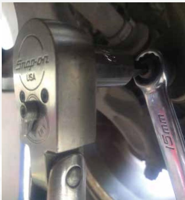
The best way to check for looseness and tighten sway bar end link nuts is to use a box or an open end wrench and hold the stud with either a Torx or Allen socket.
