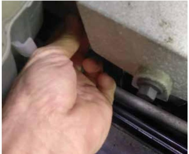
It can be very difficult to visually check the condition of the torque rod bushings while the rod is installed on the engine, since the bushings are under aluminum covers. The best way to check the bushings for wear is to just grasp the torque rod in the middle and shake it. When they are worn out the rod will rattle.
