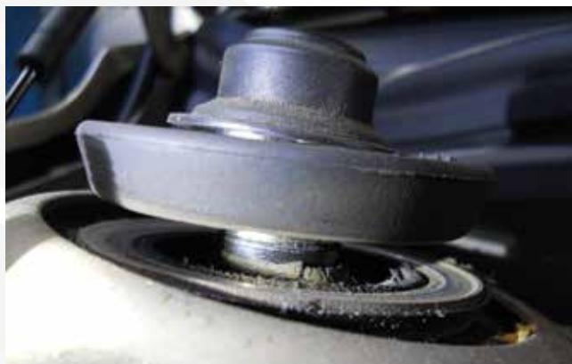
If you work on Volvo vehicles, you know what this part is and you have replaced a few broken ones. But the key is to recognize when the spring seat is about to fail and inform your customer before they hear that popping noise over bumps.
