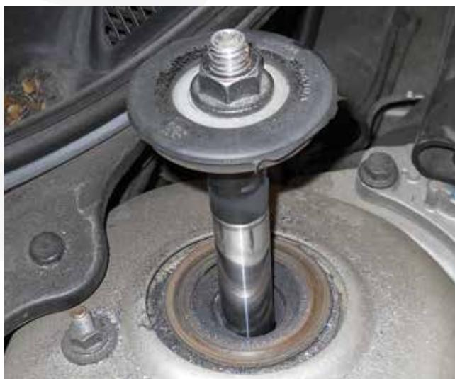
If the customer's struts are worn or have a lot of miles on them, explain to the customer that replacing the struts at the same time as the seats will save them a lot of money on labor since they have to be removed to replace the spring seats anyway.
