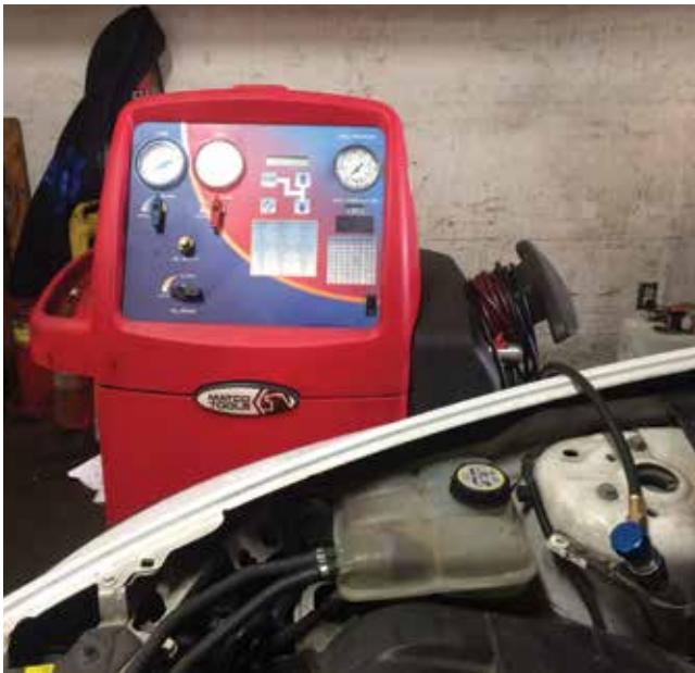
A standard A/C service console can be used to evacuate and recover the refrigerant, and for recharging the system after service is complete.
