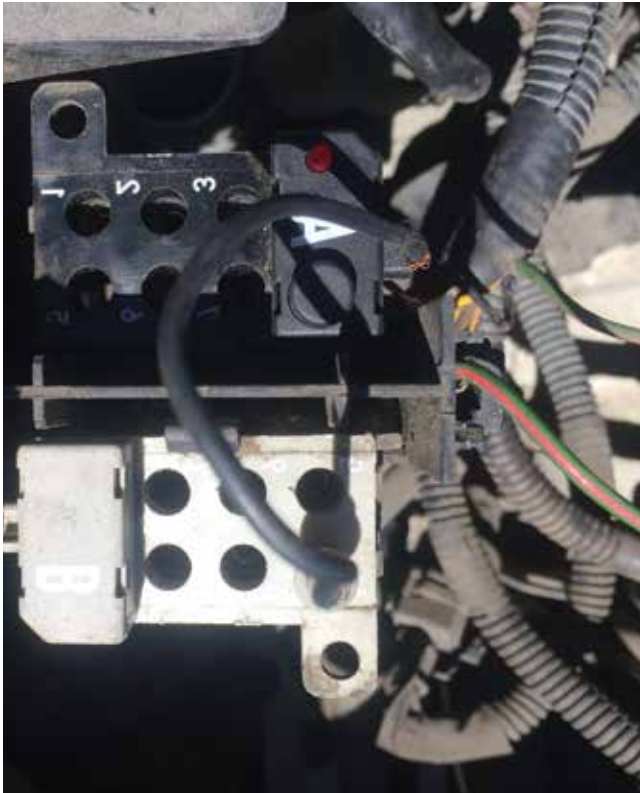
The data link is located under the hood for diagnostic purposes and for checking for fault codes in the system.
