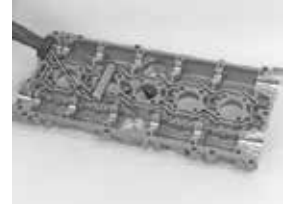
Applying Volvo sealant
