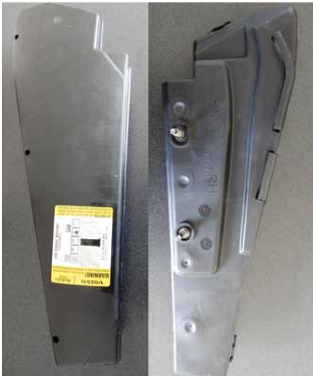
The SIPS air bag is located in the back seat and inflates from side impact.
