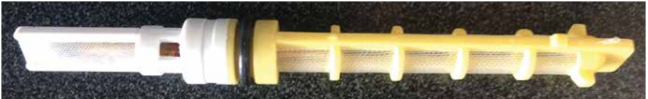
The orifice tube expansion valve is located in the high pressure hose and controls the amount of refrigerant going into the evaporator.
