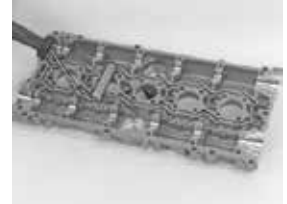
Applying Volvo sealant
