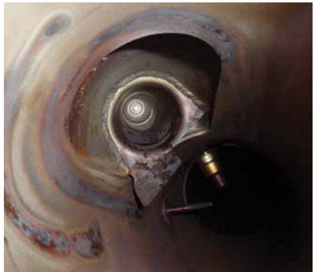
This view of the inside of the exhaust system shows just how clean BMW diesels really are! The DEF injector can be seen top left.
