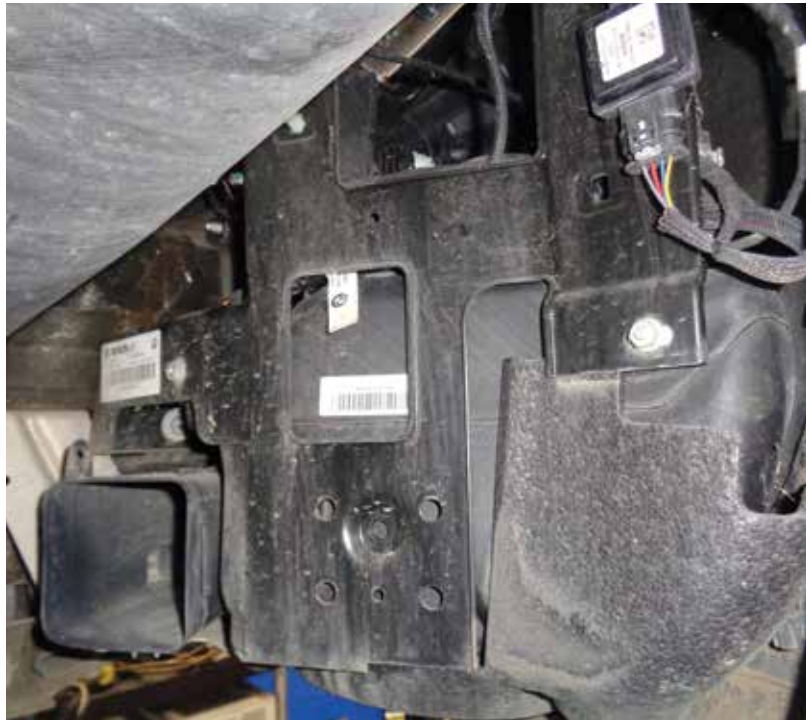
This is the active DEF tank on an E70 chassis diesel. Located in the passenger front wheel well, access is very limited without removal.
