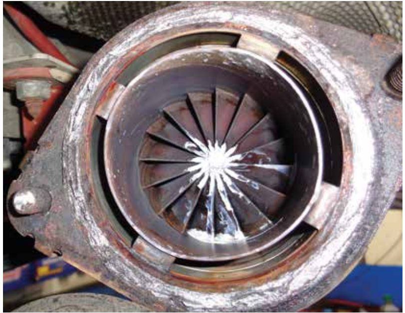
This is the "mixer" which aids in vaporizing injected DEF fluid.
