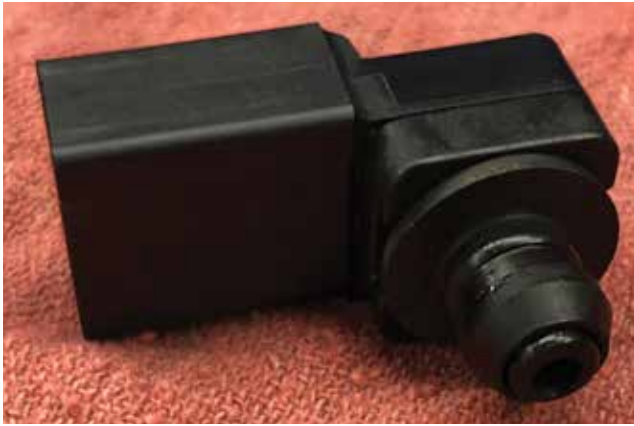
Manifold pressure sensors have a high failure rate due to fouling from carbon buildup.
