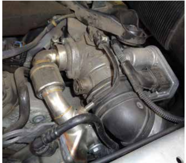
The EGR valve is mounted between the intake manifold and throttle unit. Also note the small flex pipe on the EGR. These do fail occasionally, leaking exhaust gases.
