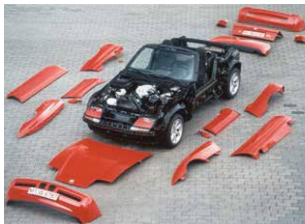
BMW has extensive experience with plastic body panels. Shown here in red are all of the plastic body panels from a 1990 BMW Z1.
