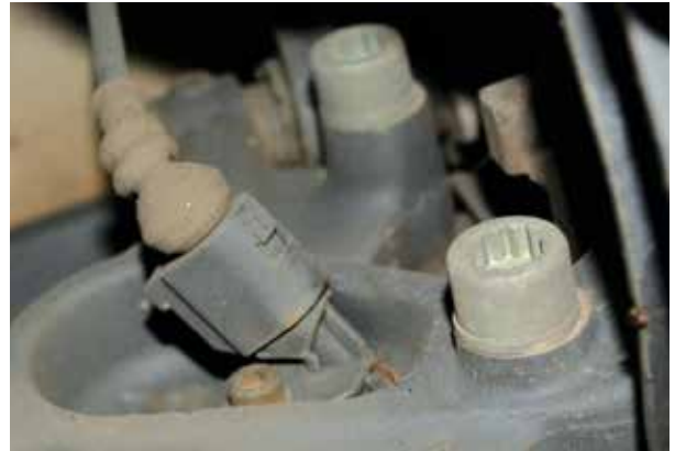
Corrosion around the base of the wheel speed sensor and its bolt can alter the sensor position, changing the air gap between the sensor and tone wheel and reducing the accuracy of the voltage signal to the ABS controller. If the sensor is undamaged, you may be able to remove it (be gentle with its plastic housing), clean the corrosion off of the mounting area, coat it to minimize future corrosion, and re-install the sensor. VW recommends using hot bolt paste (VW part number G 052 112 A3) on the mounting area for Jetta wheel speed sensors, but you should check your repair information for sealer recommendations for specific year and model vehicles.
