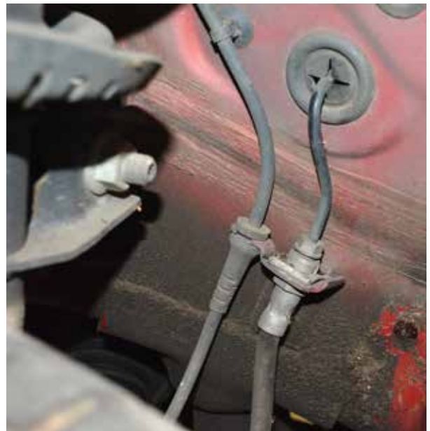
The brake hard line is more vulnerable to collision damage than the flexible brake hose, but both should be checked for leaks, cuts, or other abrasion damage.
