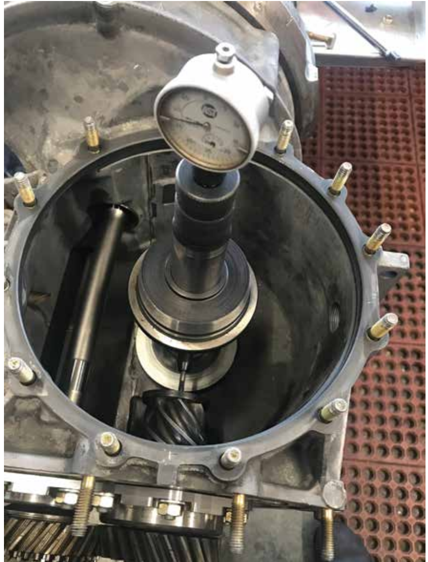
This is the tooling measuring pinion depth. The differential side cover is off for a better view.
