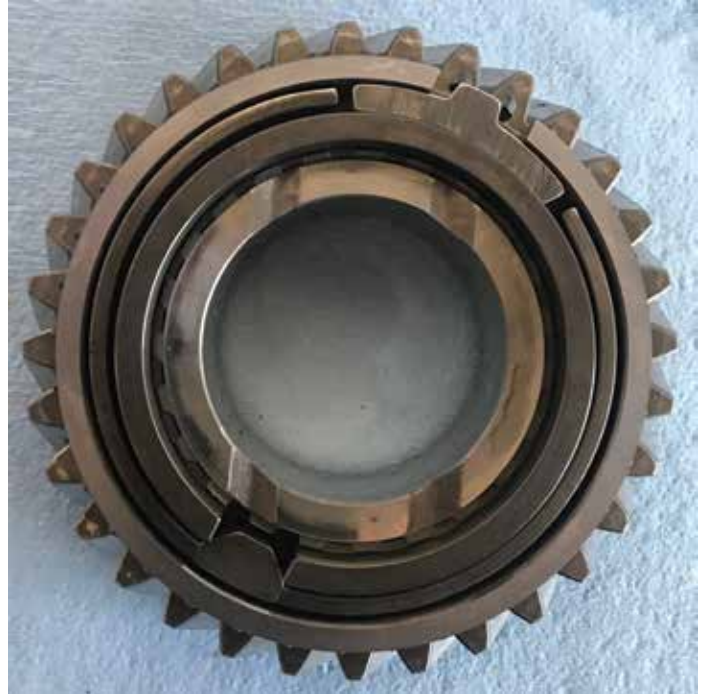
The main components of the Porsche style synchronizer are shown here prior to snap ring installation.
