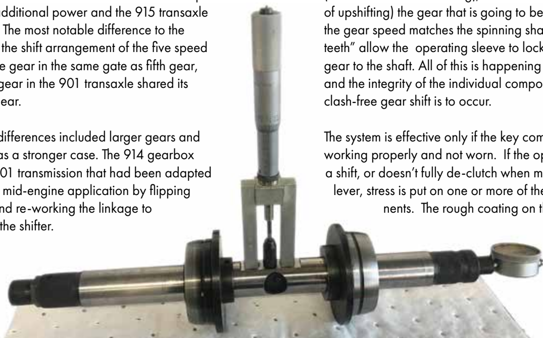
This is the setup tool for pinion gear depth being calibrated for its specific application.
