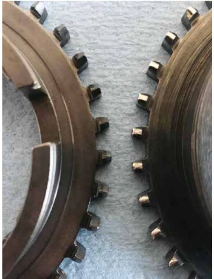
The dog teeth on the right are severely worn. Compare them to the new unit on the left.
