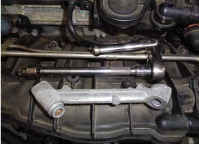
These intakes have enough problems and need all the support they can get. Don't forget to re-install this necessary brace!
