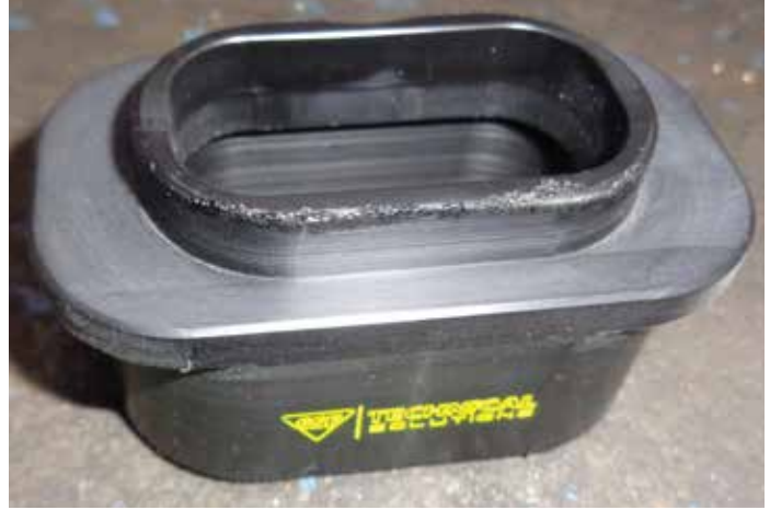
Having a well-fitting port adapter can make a huge difference in controlling unintended walnut shell dispersal.
