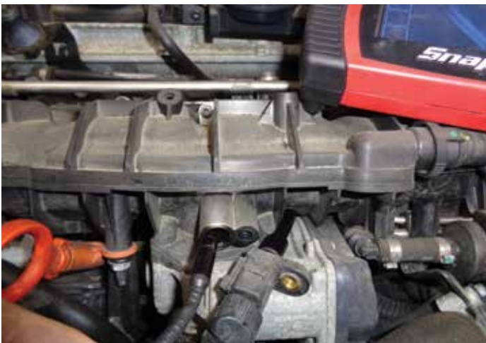
By removing the intake temperature sensor from the intake on the 2.0t engine, a borescope can be easily inserted to inspect for excessive carbon buildup.
