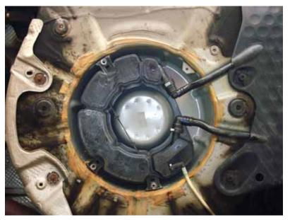
Due to space constraints, we now have some unusually-shaped canisters. This 2005 Jetta has one mounted under the trunk in the hole of the spare tire well. You can see the two large hose fittings that go to the fuel tank and refueling lines. Also, note the smaller white line that brings the vapors to the canister purge solenoid. Check all of the fittings as they are potential leak spots.
