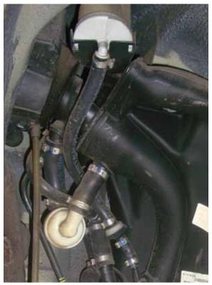
If you suspect a leak in a plastic housing such as the canister itself, or the fuel tank filler tube, you can pressurize the system without smoke and spray a soap-and-water solution and look for bubbles. Try spraying around seams first, then look at joints and hose connections.
