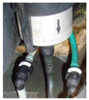
When looking for leaks, it is a good idea to check all the connections first. On this 2005 Volkswagen Jetta fuel filter, the black line is the fuel feed, the green line is the fuel return, and the white is the EVAP line from the canister to the purge solenoid. Check for proper sealing.
