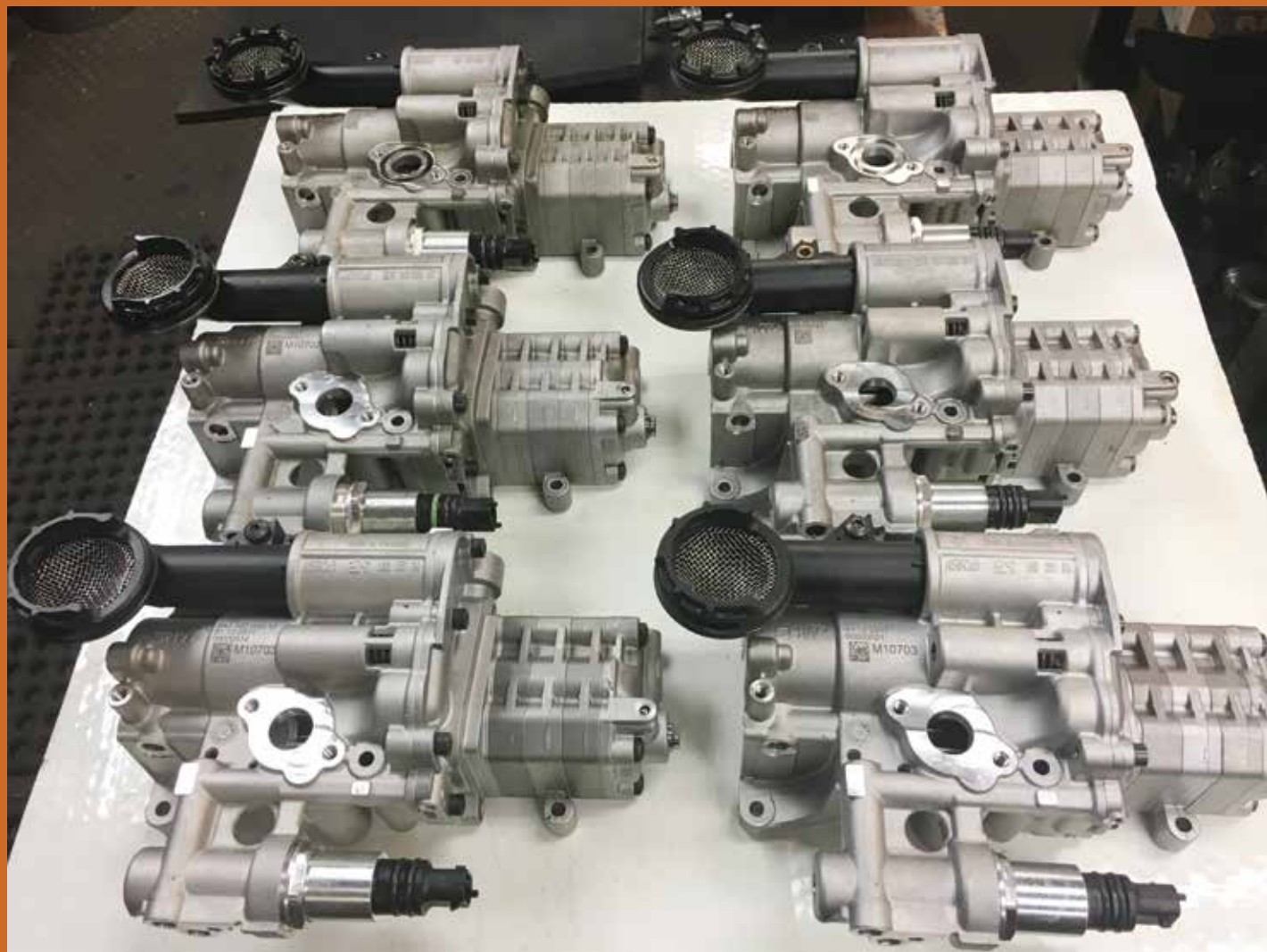
Porsche 9A1 engine Variable displacement oil pumps. First generation top left 9A1 107 050 03. To the right is updated pump 04; center row left is 05; center row right is 05 with updated control pressure solenoid. Bottom row left is the 011 pump; and to the right lower row is the most current updated pump assembly 9A1 107 050 12.
