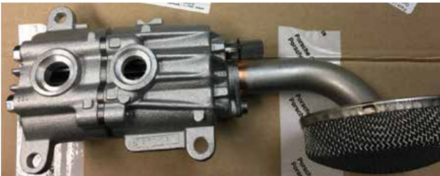
On the Carrera oil pump pictured this is a two stage pump.
