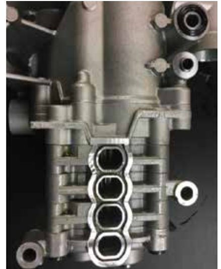
Four stage scavenge section of the 9A1 oil pump. Image on the left is the early style with viton seal. Right image is the late style pump which eliminated the four compartment seal.
