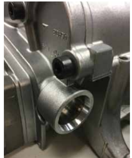
Early model 9A1 pump scavenge outlet without lock.
