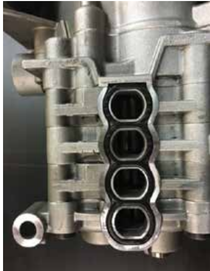
Four stage scavenge section of the 9A1 oil pump. Image on the left is the early style with viton seal. Right image is the late style pump which eliminated the four compartment seal.
