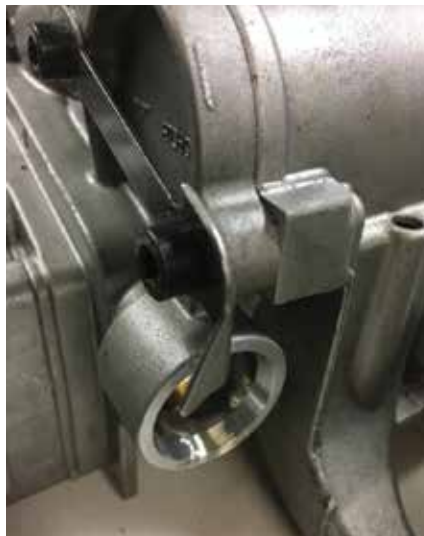
Early model 9A1 pump with scavenge discharge lock.
