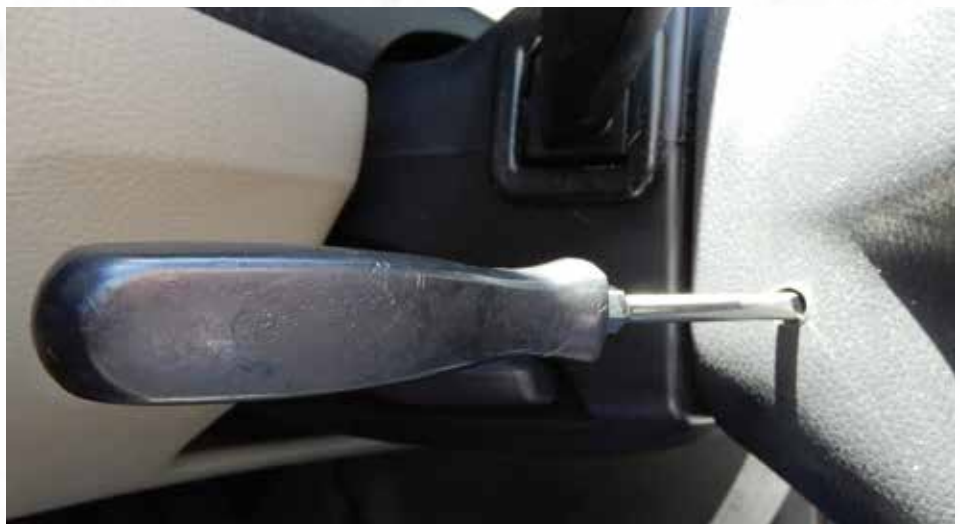
Screwdriver inserted in steering wheel to remove air bag
