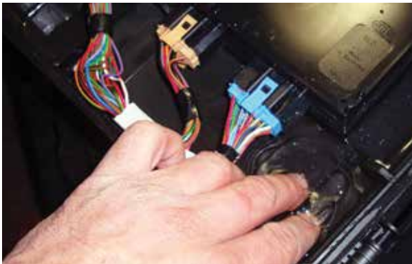
...serious water infiltration.
