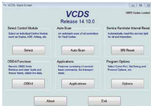
There are many “address words” for all of the possible self-diagnostic systems on the vehicle. Select address word 08 – HVAC and you can talk to an automatic climate control system (not a manual system).
