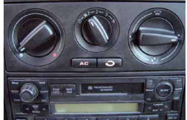
The traditional three dials of the Volkswagen manual HVAC system couldn't be simpler to understand and operate. This switch unit provides voltage to Pin #8 on the cooling fan control unit indicating that A/C has been requested.
