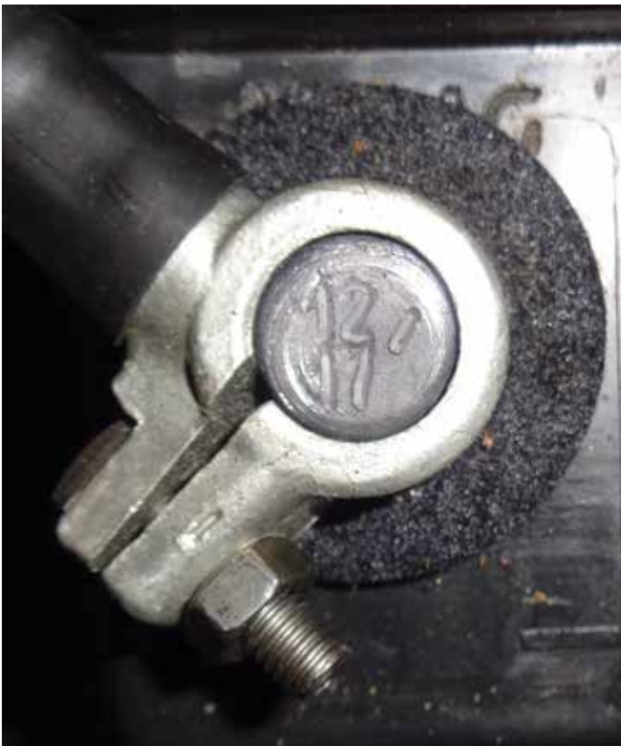
Original batteries are usually date-coded so you can quickly verify their age.
