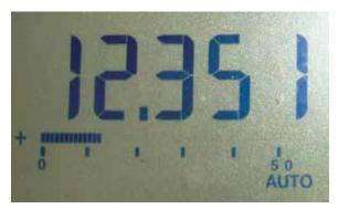
Here, we are checking the power supply to the central locking module. Battery voltage read 12.6, and here at the module and ground we're finding 12.31V.
