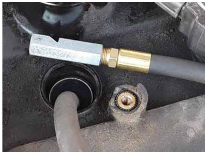
This is a TDC whistle. The most valuable inexpensive tool in the tool box. Use it to identify top dead center using the engine's compression. Warning, if your valve timing is off it may not be accurate.
