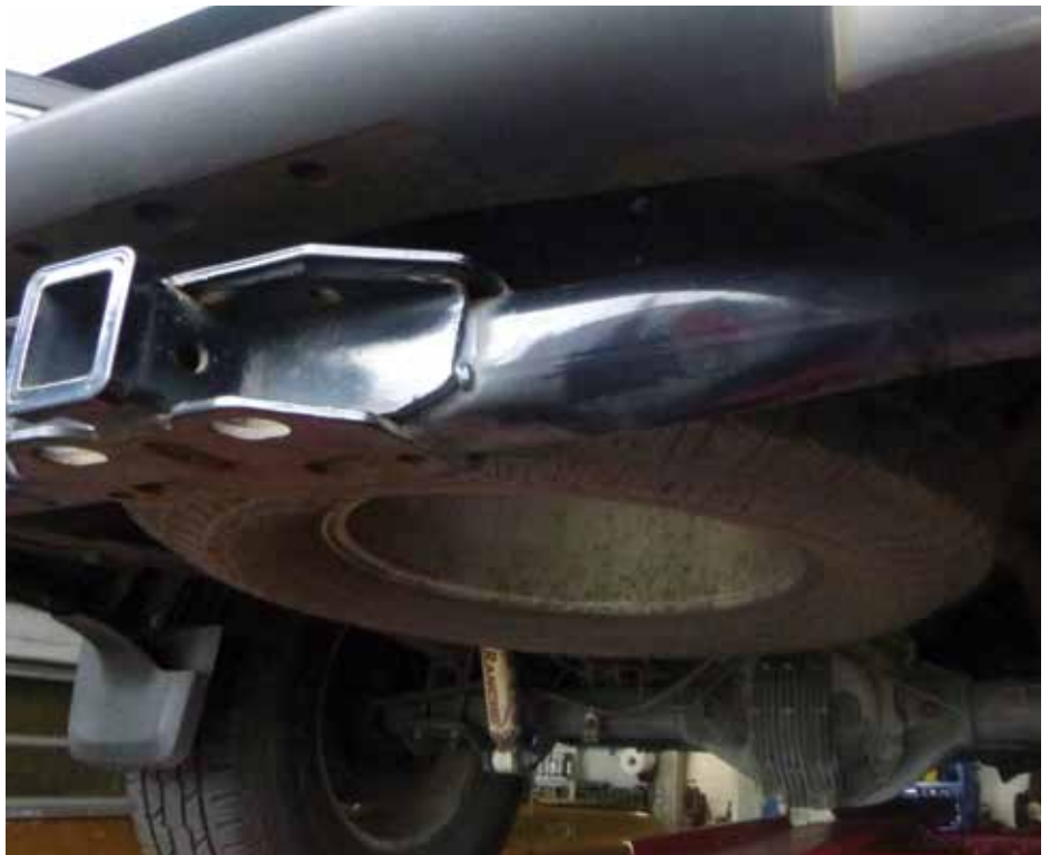
The presence of a factory trailer hitch receiver may indicate the truck has the factory towing package that comes with a shorter gear set to improve performance while towing heavy loads.
