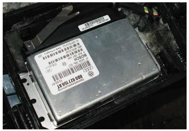
On Passats from the late '90s and early 2000s, the TCM is mounted under the carpet on the passenger side. In this case, water from leaking seals has collected under the carpet and corroded the connector for the TCM. This can cause harness-related DTCs.
