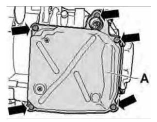
The Mechatronics unit is mounted behind a cover plate and is immersed in transmission fluid. This fluid must be drained before accessing the Mechatronics unit.
