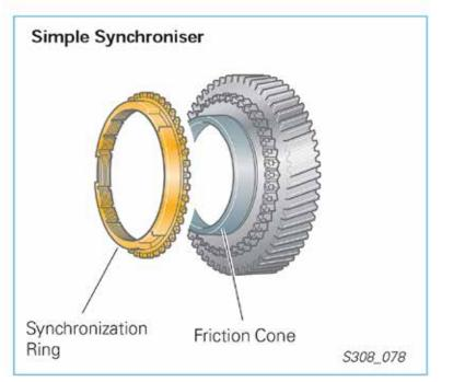
The triple synchronizer is used on the first, second, and third gears; the single synchronizer is used on fourth, fifth, and sixth gears.
