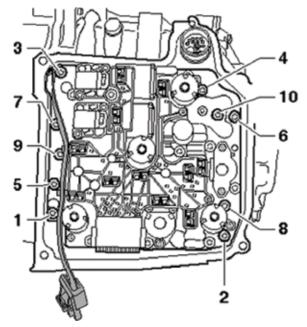
The Mechatronics unit is mounted with ten bolts which must be removed and installed in sequence. These are single-use bolts and must be replaced at every service.
