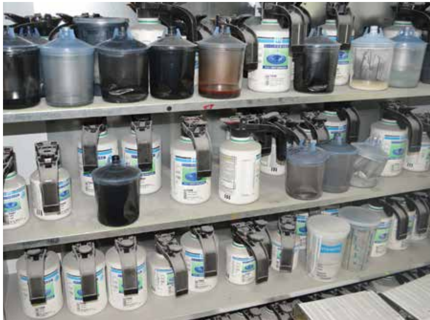
Store and mix water-based paints only in plastic or inner-coated tin containers to avoid corrosion contamination problems.
