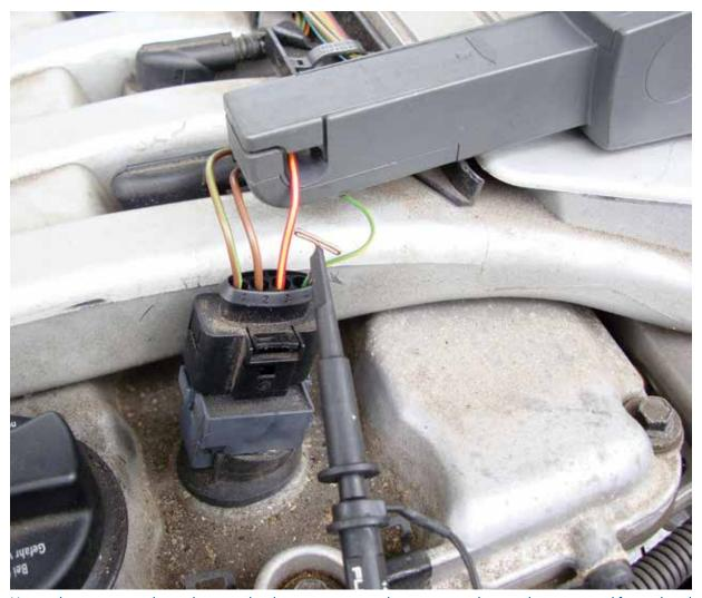
Using a low-current probe and a scope lead, you can monitor the amperage draw and trigger signal for each coil you are testing. Here, we've used the wiring diagram to identify the power supply wire and the coil trigger. We put the current probe around the power supply and back-probed the coil trigger with the scope lead.
