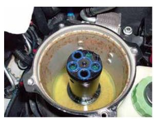
Rust in the fuel system causes rough running and a possible no-start, according to VW TSB #2023624/2. Debris and sludge can plug the fuel filter and cause the system to set a DTC POO87 – Rail Fuel Pressure Too Low.
