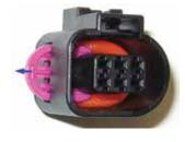
harness end connector housing to allow secure insertion of wire terminals. The repair corrects a corrosion-related contact resistance fault in the ECM wiring for the throttle valve.
