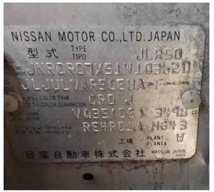
Found on the right side of the bulkhead (firewall), this ID tag has all the information you need, including VIN, engine, transmission, and axle information, making ordering the right parts an easy task.
