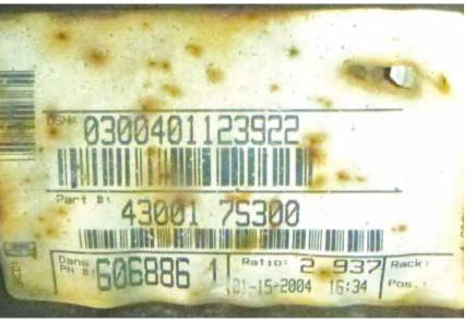
With the identification sticker intact, this axle won't be difficult to correctly identify. The gear ratio of 2.937:1, the part number, and even the original Dana part number are all right there for you. Too easy.
