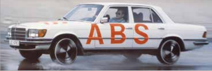
The 1978 S-Class (model series 116) was the first production passenger car in the world with ABS.
