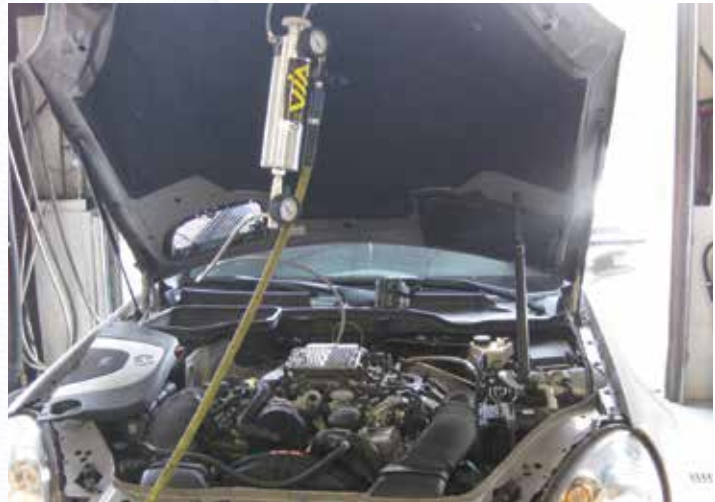
This vehicle has an intermittent p2004 code, meaning the intake runner flap on bank 1 is sticking. The chemical cleaning procedure may be too late.
