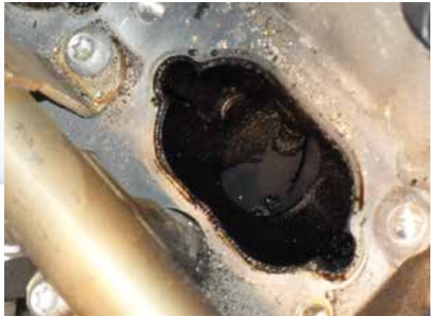
Carbon build-up can be huge, and very detrimental to performance
