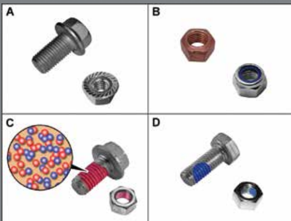
Mercedes-Benz uses four basic types of single-use fasteners: A. Locking splines B. Self-locking nuts C. Microencapsulated screws and nuts D. Polyamide coating. Types A, B and C must always be replaced after they have been used. Type D can be re-used if not damaged unless specifically prohibited in WIS. Be sure to review the WIS document AH00.00-N-0001-01A for an explanation of how to recognize and work with these fasteners.
