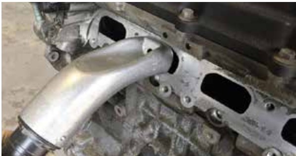
You may need to modify the adaptor to prevent blow-back of the media.
