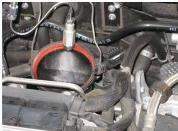
A super-fine solvent spray mist can be introduced into the throttle body to clean the intake tract. It’s sensible maintenance.
