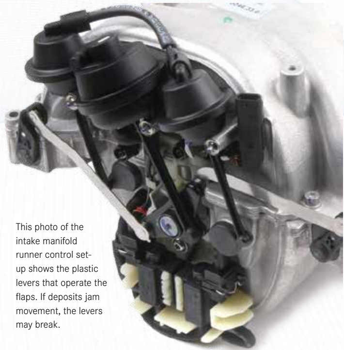
This vehicle has an intermittent p2004 code, meaning the intake runner flap on bank 1 is sticking. The chemical cleaning procedure may be too late.
