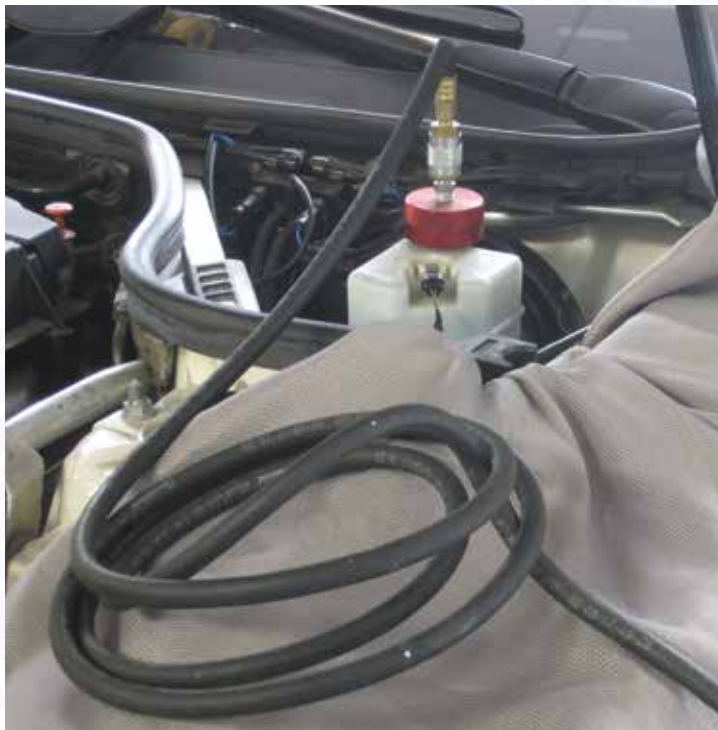
Make sure you have the proper pressure bleeding hook up before you start.
