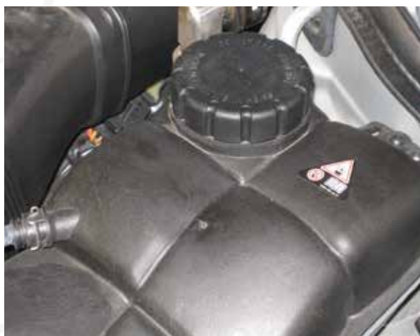
For many decades, cooling systems have been pressurized by the use of a cap that determines the psi at which it vents.
