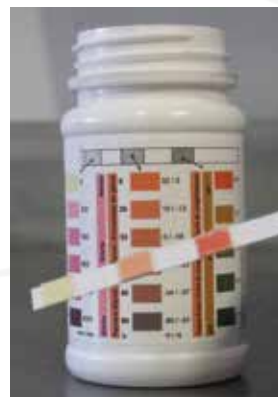
Using coolant test strips will tell you the condition of the antifreeze/water mixture.
