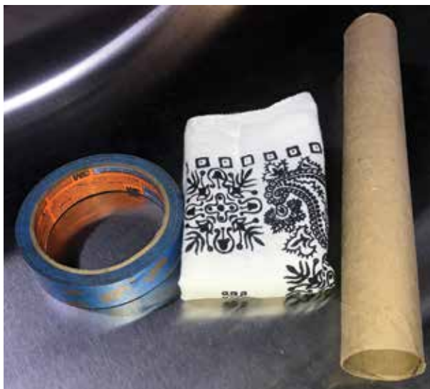
These are your basic tools for locating air and water leaks. The text explains how they're used.
