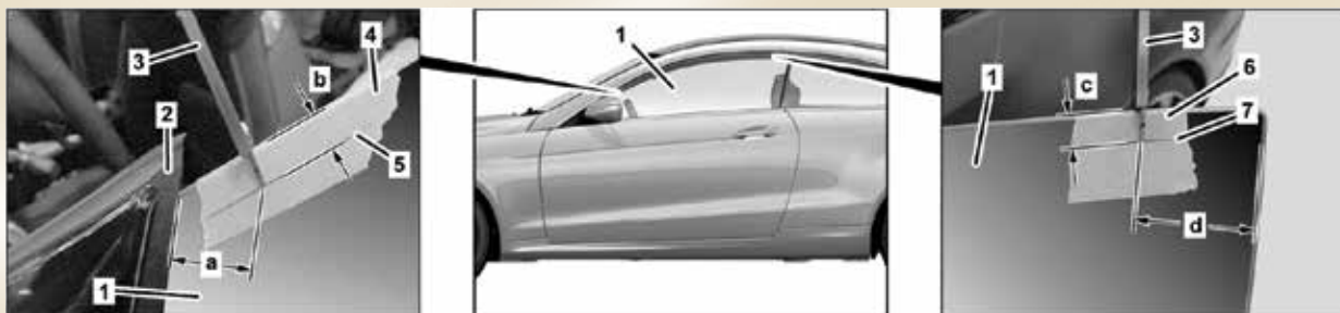
The Basic setting. Measure the distance "a" from the rear of the window to the metal edge of the door, and adjust to the specification.
