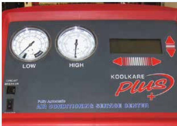
Any AC recovery/recharging machine also does leak testing.
