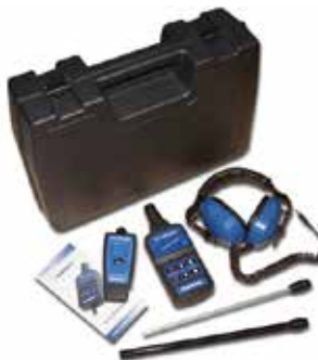
The Mercedes-Benz recommended ultrasonic leak detection tool. This kit comes with an ultrasonic transmitter and receiver, along with a headphones and a variety of probes to simplify leak locating without needing a test drive.
