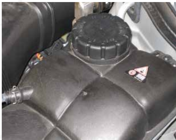
For many decades, cooling systems have been pressurized by the use of a cap that determines the psi at which it vents.
