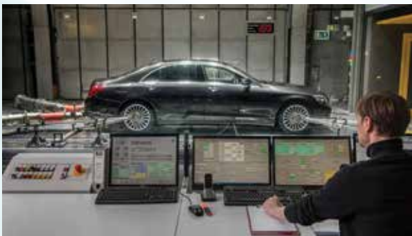
Testing a new Mercedes-Benz equipped with a CO 2 -charged AC system
