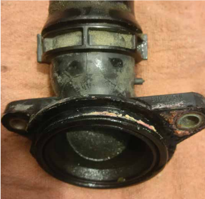
Pressure fit o-ring on edge
