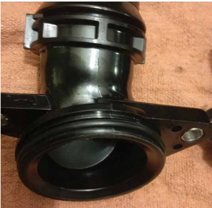
New housing with o-ring in groove
