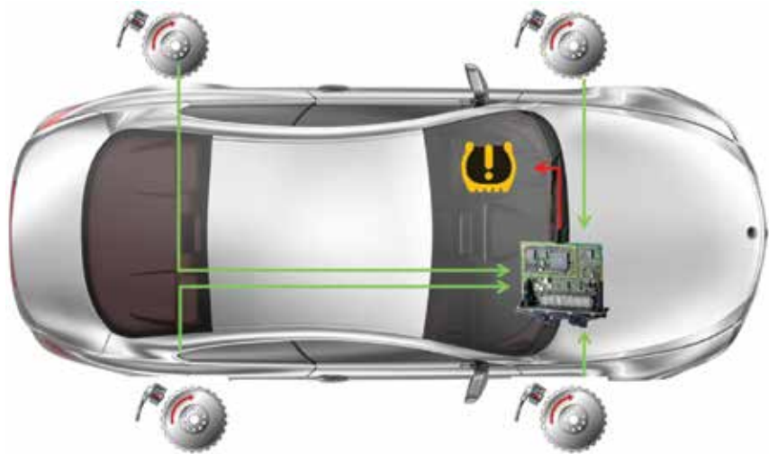
Early indirect systems relied on existing hardware: wheel speed sensors. When a tire gets low, its diameter is reduced so it takes more revolutions to cover the same distance. TPMS electronics can detect the difference and signal the driver (courtesy Hella).
