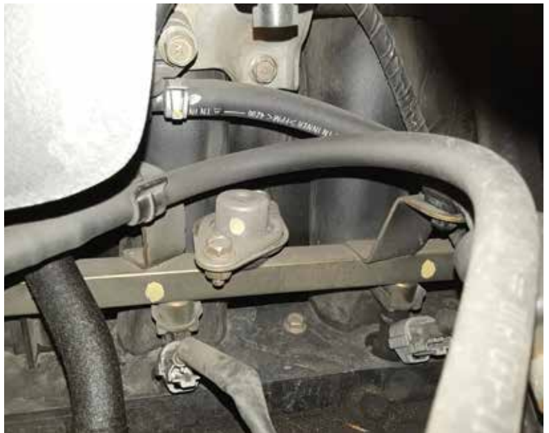
This is a fuel pressure damper in a Titan V-8. Failures are often manifested as fuel leaks. No matter how minor the leak, replace the failed damper and make it a priority.
