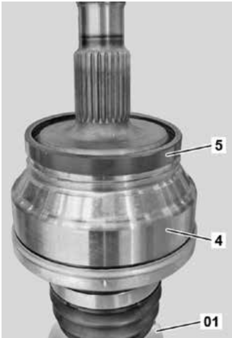
The rear axle pulse wheel (5) must be pressed on to the axle (4) and never hammered, or it can be damaged.
