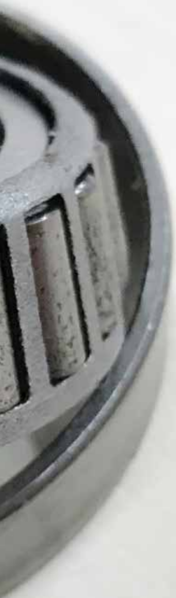
A non-adjustable rear wheel bearing integrated with the hub (10). Installation is a simple bolt-on operation once the carrier (7) is accessed.
