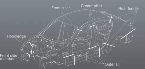
The sectioning locations marked on this image are general suggestions only. Partial repair of key structural components may or may not be allowed depending on the vehicle model's body structure, the component's material type and strength, the part's shape and internal structure (ducting, complex support, or baffles, etc.), and other factors.
