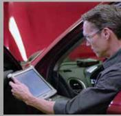
Nissan recommends using the OEM scan tool CONSULT III Plus to perform pre- and post-repair diagnostic scans and calibrations.
