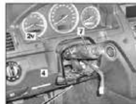
The electronic steering lock is attached at the steering column.
