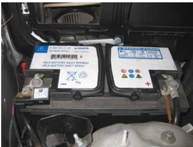
Note the amp hour rating and the IBS at the negative cable of this Mercedes-Benz battery.
