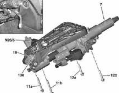
Here's the steering lock breakdown from WIS document AR46.10-P-0910CW.
