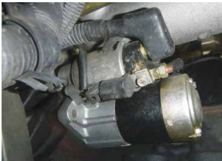
Activating the starter manually on the vehicle is as easy as applying power to the solenoid at the switch connection (the Phillips head bolt here). Use all due caution as this will, if everything's working right, crank the engine immediately.
