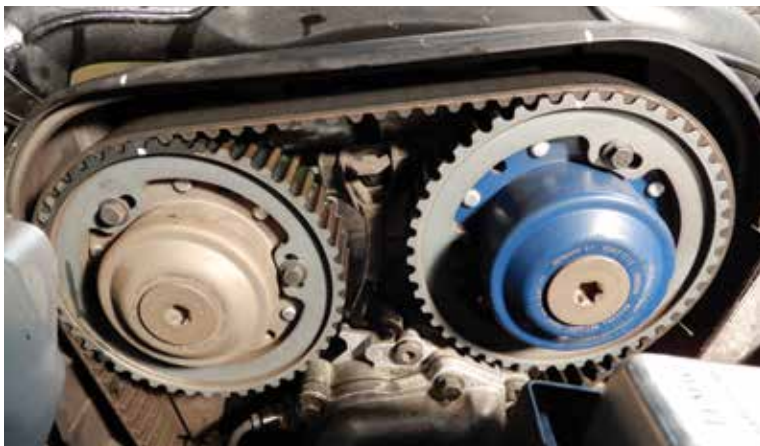
Variable valve timing units on front of camshafts and timing marks lined up with top timing cover
