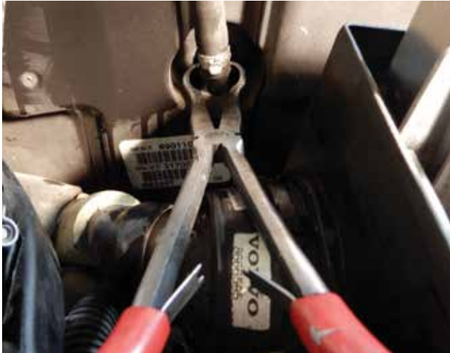
Use the correct pliers and pull out to remove hose.
