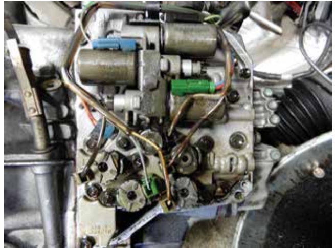
Valve body from inside transmission
