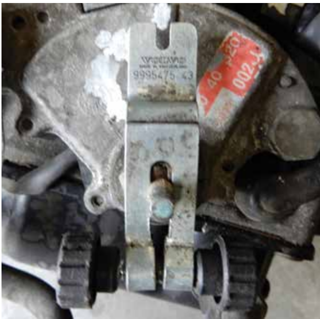
Tool installed and aligned properly on the transmission.
