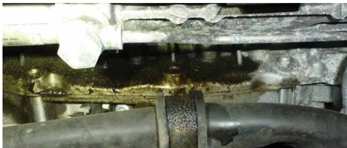
This oil leak could be from a number of different engine components; get out your mirror!
