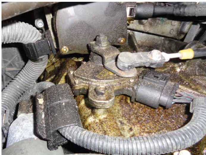
This VW 2.5L vacuum pump had covered half the engine and transmission in oil.
