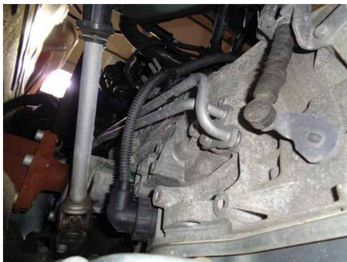
Here you can see the axle shaft, steering coupler, and most of the transmission connections that must be disconnected during trans removal.
