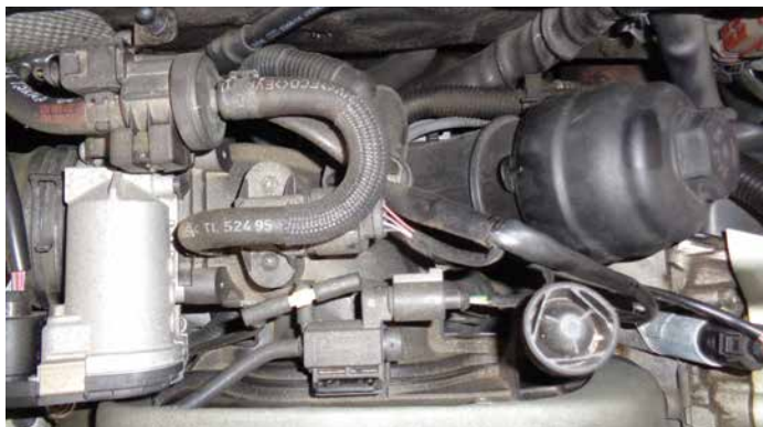
Always replace all the associated oil filter o-rings during service. You don't want a leak from the filter housing!
