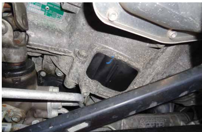
This lower cover is also used to access the torque converter fasteners.
