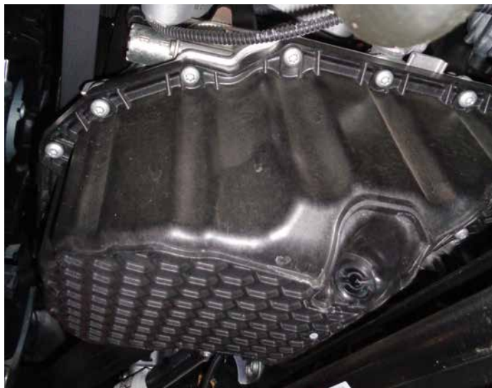
Many new Audi's have a plastic oil pan; it would not be a good idea to use a floor jack on these.
