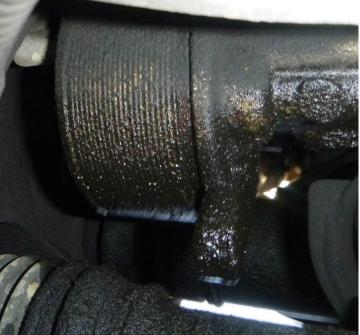
This leaking oil cooler drips a quart of oil in about 500 miles and is the cause of a recurring P0011 valve timing performance code. Low oil levels prevent the VVT from performing properly. To keep the code from coming back the oil leaks have to be found and fixed.
