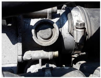
This air intake tube is folded where it meets the throttle body. This allows unmetered and unfiltered air into the engine. It's an easy thing to cause and an easier thing to miss. Did you already fix your air control problem then accidently cause another by folding the air tube?
