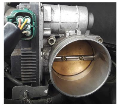
The advent of the electronically controlled throttle body brings engine control to a new level. Is it any surprise that the diagnostic procedure is just as complex?
