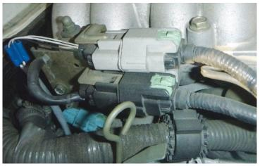
The upstream oxygen sensor connectors are right next to each other on the top of the engine, making diagnosis easier but making it possible to confuse the two sensors. Notice the solderless butt connectors, indicating an aftermarket universal part. Although not ideal, it should still be tested before condemning it.
